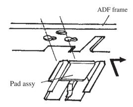
NOTICE: Pad can be replaced by aligning the holes of the pad with the pins of the Pad holder.
